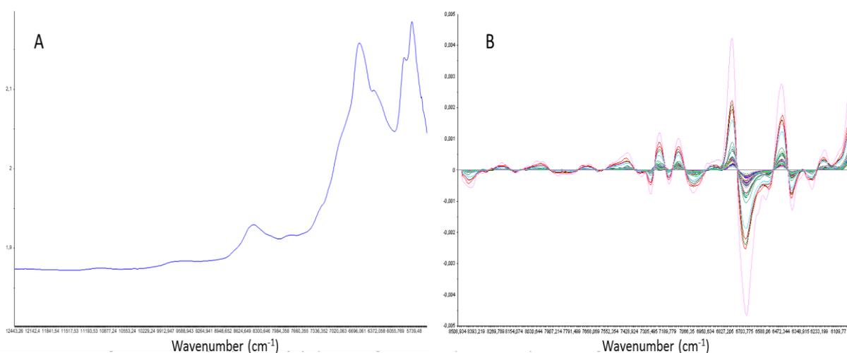
Figure 4 : A – Average spectra of lyophilized gelatin samples (5500-12500 $\text{cm}^{-1}$ ), B – Second derivate and smoothing spectrums of lyophilized gelatin samples (6000-8500 $\text{cm}^{-1}$ )
