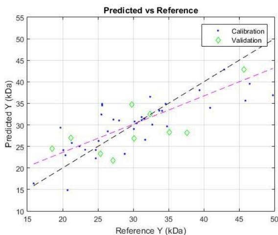
Figure 6 : Mn determined by NIR plotted against reference values for average Mn of extracted gelatin
