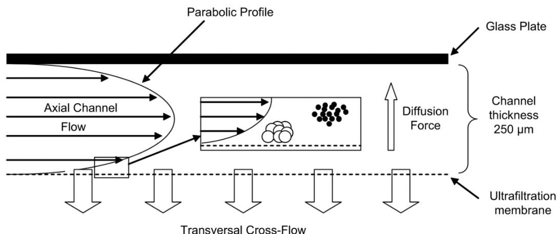
Figure 1 : Separation of samples in AF4 (● small sample component; ○ large sample component) (Rbii, 2010)
