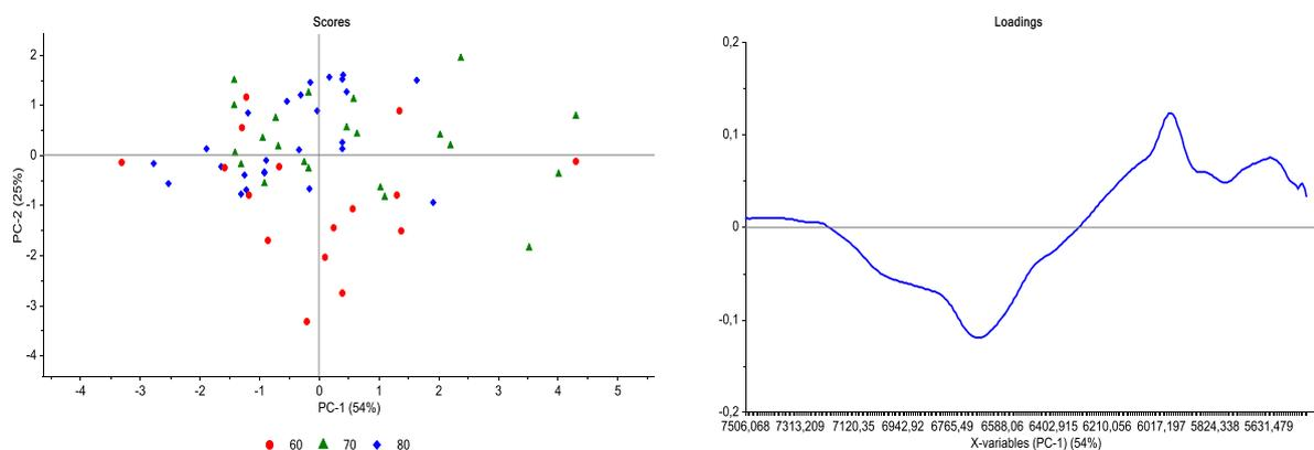
Figure 3 : PCA results (scores for PC1 and PC2, loadings of PC1) for gelatin over the 5800–7500  $\text{cm}^{-1}$  range.
