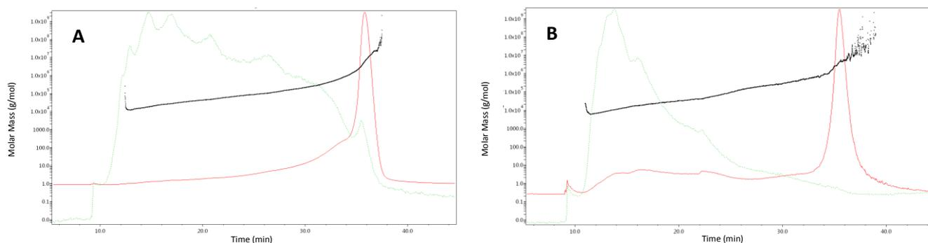
Figure 2 : Fractograms from gelatin samples: (A) sample extracted at 60 °C after 4 h, (B) sample extracted at 80 °C after 12 h. Transmitted UV intensity (green dotted line) and light-scattering intensity (red solid line) are expressed in arbitrary units. The calculated molar mass is represented by the black dots.
